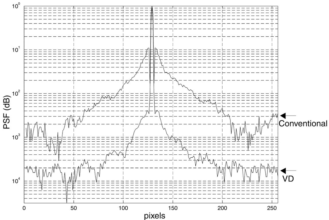
FIG. 3. Cross sectional plot of the simulated point-spread function for variable density (VD) and conventional spiral designs. A simulation of the point-spread function. The middle slice profile is given for the reconstructed impulse function. Side lobes are reduced for variable density (solid) acquisition compared to conventional spirals (dashed) while nominal resolution and SNR are the same.
