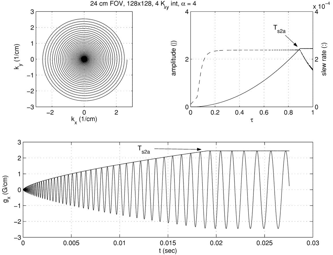
FIG. 2. Design example of a four interleave,  $128 \times 128$  resolution, 24 cm FOV variable density spiral trajectory using gradient characteristics of amplitude: 2.2 G/cm, slew rate: 25 G/cm/ms. Corresponding  $k$ -space trajectory, amplitude, and slew-rates and gradient values are given.
