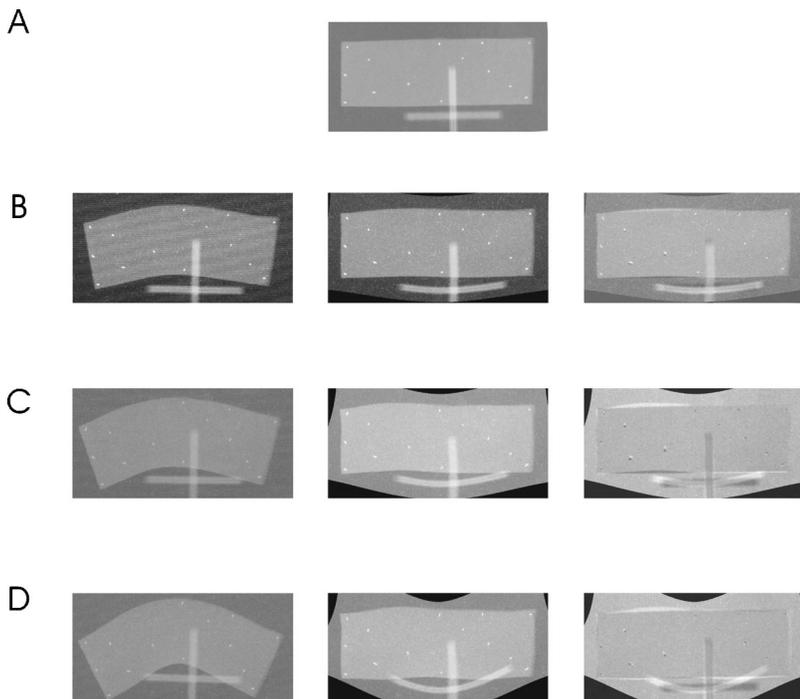
FIG. 3. A registration study by systematically bending a rectangular phantom. (A) The original phantom. (B) The distorted phantom (left), the TPS-warped phantom (middle) and the difference image between computed and original one (right). (C) and (D) are similar to (B) except with increased distortions.
